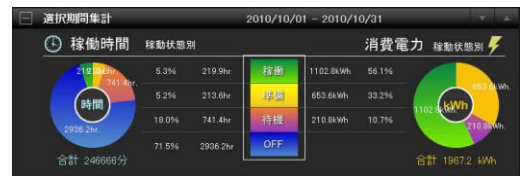
図 16 Gr-Value Bee 電力と時間の集計グラフ Fig.16. Gr-Value Bee Summary of power consumption and time
